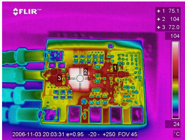
Figure 11a – Temperature Distribution, Top side
